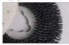
Three quick-release Tynex abrasive brushes, rotating between 350 and 700 rpm, easily strip a 51cm width.
